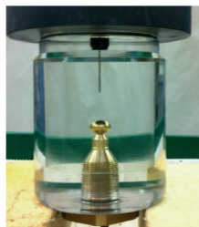
Needle - sphere (IEC 60897 method A) 300 ml oil Steel needle tip radius 7.2 micron ellipse Brass sphere electrode 12.5 mm diameter
